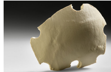
PEEK Vestakeep® i2 G cranial implant Biocompatible and biostable High installation space temperature (~200°C)
