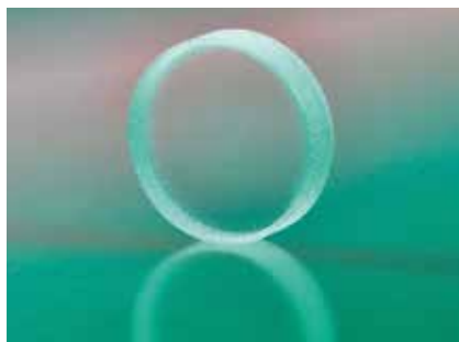
Fig. 6. If the droplets are extremely densely packed, transparent test plates made from PMMA can be manufactured using the APF process (© Arburg)
