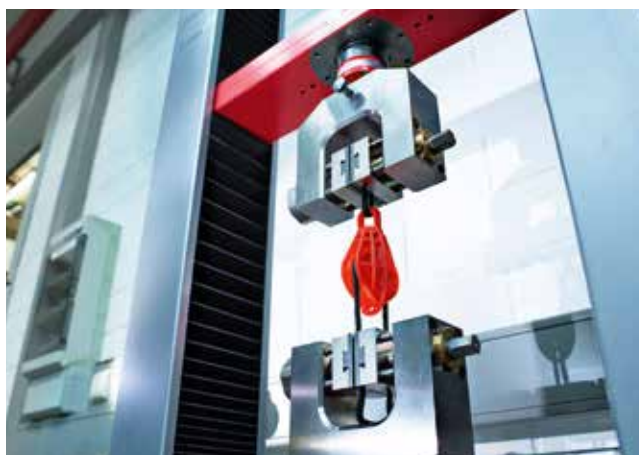
Fig. 9. Complete module additively manufactured in a fully assembled state: an articulated rope pulley made from bio-PA has a load-bearing capacity of 100 kg (© Arburg)
