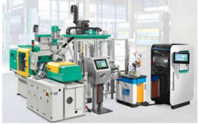
Fig. 14. In a fully IT-networked and comprehensively automated production line for individualized high-volume parts, a seven-axis robotic system is used to feed the build chamber of the Freeformer (© Arburg)
