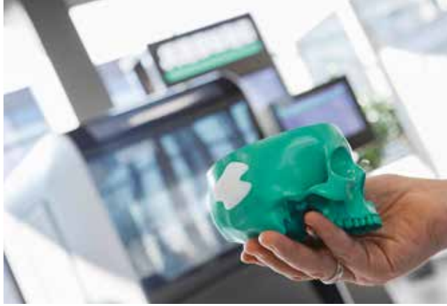
Fig. 10. By way of example, a Freeformer produced an individually adapted cranial bone implant made from medical grade PLLA granulate (© Arburg)
